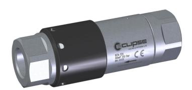
A system is limited by its most restrictive component, which is why couplings with high flow capacity are so important. Eclipse breakaways allow operators to fully utilize larger bore hoses and couplings without constricting the flow with an undersized breakaway. Especially designed for high flow NGV filling such as trucks, buses and mobile storage units.
